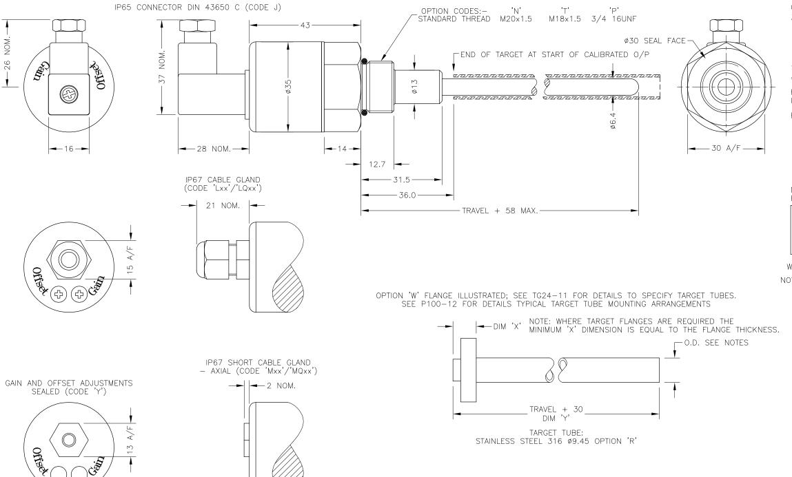
ELECTRICAL OPTIONS/ SPECIFICATIONS <u>OUTPUT</u> **SUPPLY** 0.5 TO 4.5V RATIOMETRIC 5V SUPPLY CURRENT 12mA TYP. 20mA MAX. CABLE:  $0.2 \, \text{mm}^2$ , 0/A SCREEN, PUR JACKET — SUPPLIED WITH 50cm OR REQUIRED LENGTH IN cm (15000cm MAX). STANDARD 3-CORE: JACKET Ø4mm BLACK e.g. 'L50' OPTIONAL 5-CORE: JACKET Ø4.6mm BLUE e.g. 'LQ50' CABLE/CONNECTOR\* CONNECTIONS; 5 CORE CONNECTOR 3 CORE RED RED ORG +SENSE (5-WIRE ONLY) BLACK BLACK OV GRY -SENSE (5-WIRE ONLY) WHITE WHITE OUTPUT SCREEN SCREEN BODY
